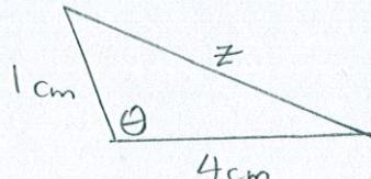
$$\begin{aligned} z^2 &= (1 \text{ cm})^2 + (4 \text{ cm})^2 - 2(1 \text{ cm})(4 \text{ cm}) \cos \theta \\ &= (17 - 8 \cos \theta) \text{ cm}^2 \end{aligned}$$
